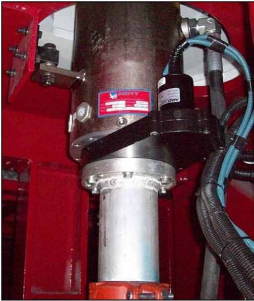
Figure 6 Amity Swivel with AMCI DuraCoder
